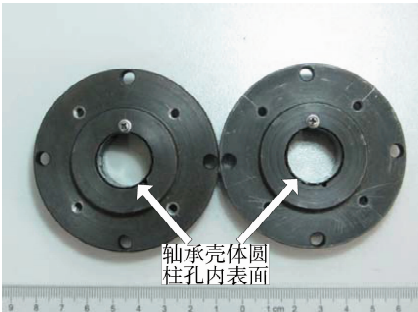
图 3 不同轴承壳圆柱孔内表面表面粗糙度的波箔型径向气体轴承 Fig. 3 Bump foil journal bearings with different surface roughness of bearing housing cylindrical hole surface
